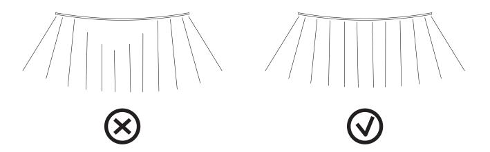
Place downwards with both hands at the edges of the linear brass and bend down until the light effect is even.
