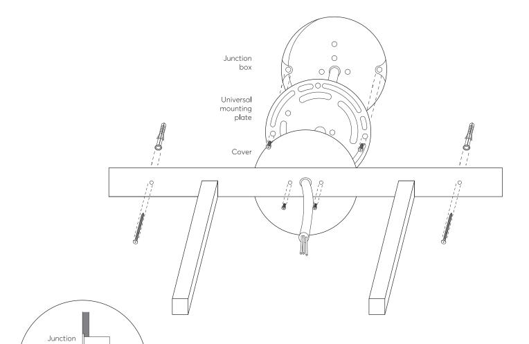
Install the junction box, pull the cable out of the central hole and screw the universal mounting plate onto the junction box. Screw the wall metal bracket on the wall.
