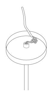
Adjust the ceiling rose at the metal bracket by using the hex (allen) key.
