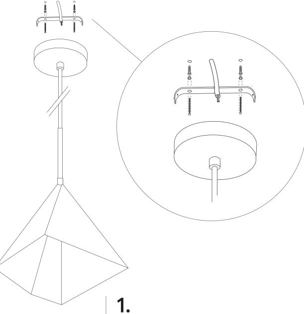
Fix the bracket up at the ceiling.
