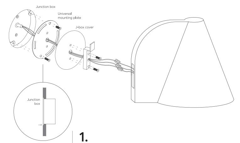
Install the junction box, pull the cable out of the central hole and screw the universal mounting plate onto the junction box.
